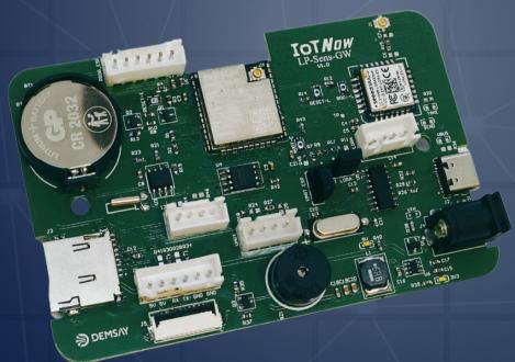
LPKIT-Gateway is a low power consumption and long range communication solution developed for industrial IoT and data monitoring applications. It provides point-to-point communication with LPKIT-Sens over LoRa protocol and makes incoming data viewable on DWIN Smart Screen via UART connection.,
